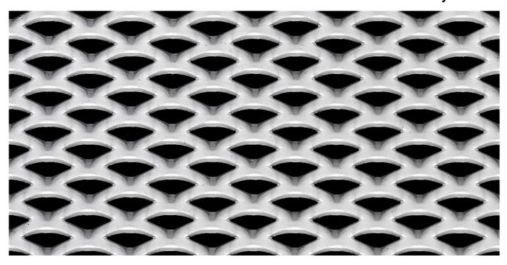
LW Pitch:30.48mmStrand Width:4.75mmSW Pitch:12.70mmThickness:2.50mmWeight:14.68 kg / m2Open Area:25%
